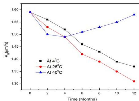
**Figure1** Variation of Bulk etch rate with Time at different temperatures.
