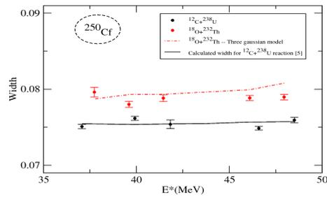
FIG. 4: Width of fission-fragment mass distribution vs  $E^*$ (MeV). The red dash-dotted line is three gaussian model prediction for non-CN reaction.
