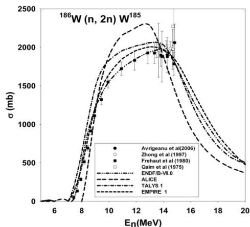
Fig. 1: Excitation function of  $^{185}\text{W}$  from  $n + ^{186}\text{W}$
