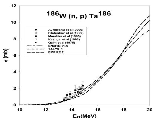
Fig. 2: Excitation function of  $^{186}\text{Ta}$  from  $n + ^{186}\text{W}$
