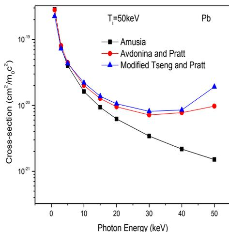
**Fig.1** Plots of total bremsstrahlung cross-section versus photon energy at incident electron energy of 50keV for Pb.
