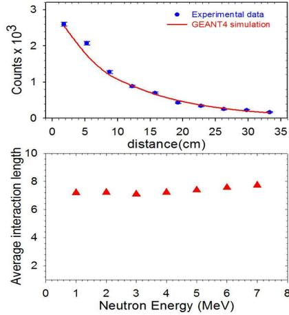
FIG. 2: [Top panel] Variation of the number of events as a function of distance corresponding to the number of detectors. Filled circles are the experimental data points and continuous line represents GEANT4 simulation. [Bottom panel] Average interaction length vs neutron energy.
