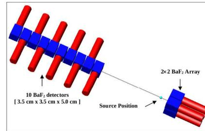
FIG. 1: Experimental set-up for the measurement of average interaction length of neutrons in BaF<sub>2</sub> material.
