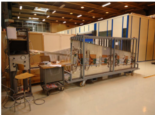
Fig.3, A Super Module Assembly under leak test for cooling sets at 904, CERN
