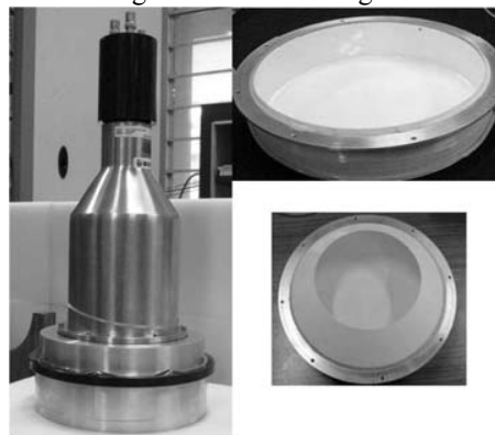
Fig. 1 Photograph of the MONSTER cell. The detector was thoroughly tested using standard \gamma and neutron sources. The pulse shape discrimination (PSD) property of the detector
