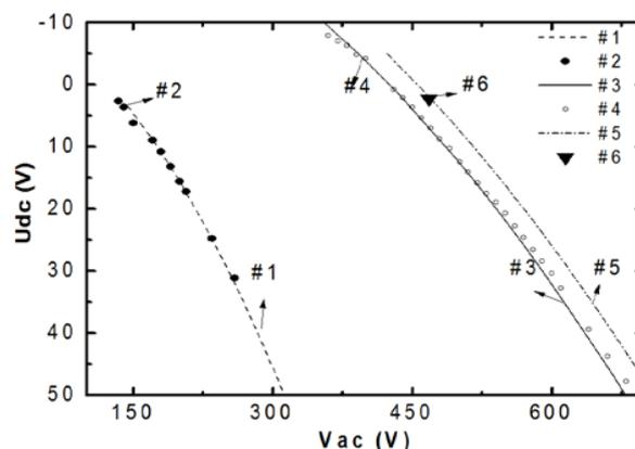
Fig 1. Plot of the equi-frequency lines in terms of applied voltages, for  $^{39}\text{K}^+$  (Theoretical #1, Experimental #2),  $^{138}\text{Ba}^+$  (Theoretical #3, Experimental #4),  $^{146}\text{Eu}^+$  (Theoretical #5, Experimental #6).
