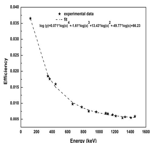
Fig. 1: Efficiency calibration curve as a function of gamma energy.
