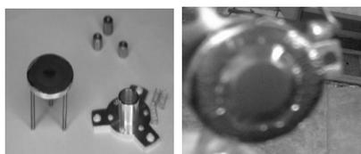
Fig. 4: Frame and cone of plunger device before stretching and after stretching.
