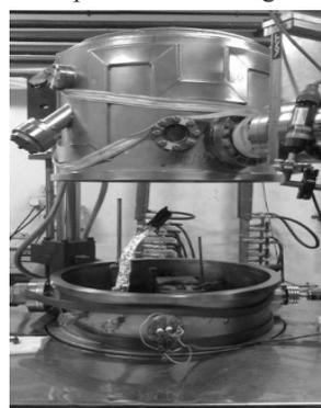
Fig. 2 : A picture of UHV evaporator in open position.
