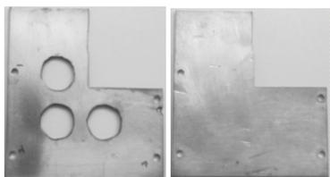
Fig. 3: Two parts of a New Substrate Holder.
