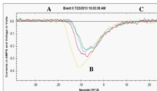
**Fig. 1** A few typical pulses recorded in the oscilloscope (1000 points: 0.8 ns/bin)
