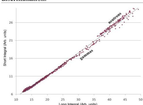
Fig. 2 A simple pulse shape discrimination plot
