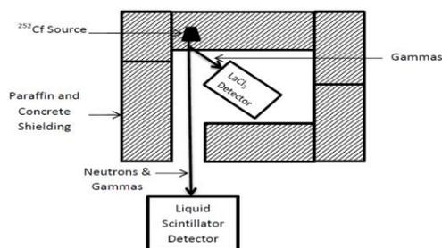
Fig.3. The TOF setup
