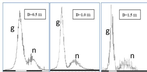
Fig.4. The shift in the neutron TOF peak with increasing source-detector distances (D=0.5, 1.0 and 1.5 m).
