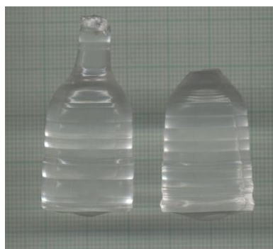
Fig. 1 As-grown single crystal of LGBO:Ce crystals.
