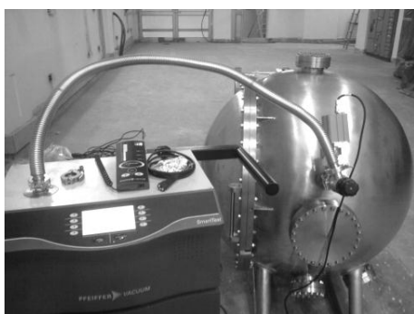
Fig. 2. One meter diameter target chamber.
