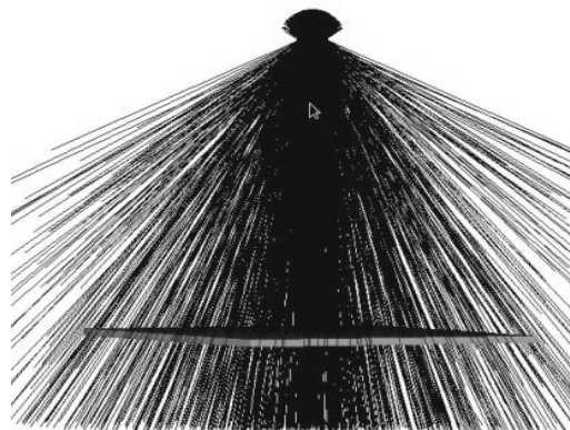
FIG. 2: A simulated diagram of cosmic ray muons passing through one RPC detector at sea level.
