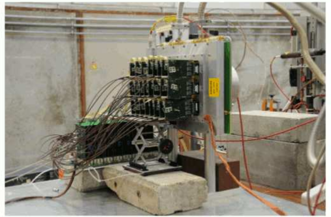
FIG. 1: RICH prototype at the PS/T10 beamline at CERN.
