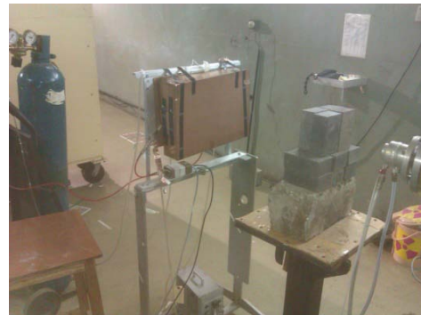
Fig. 2 Picture of the neutron test setup at VECC. Top picture shows the setup with beam shielding.
