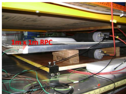
Figure 1: RPC with Scintillator paddles
