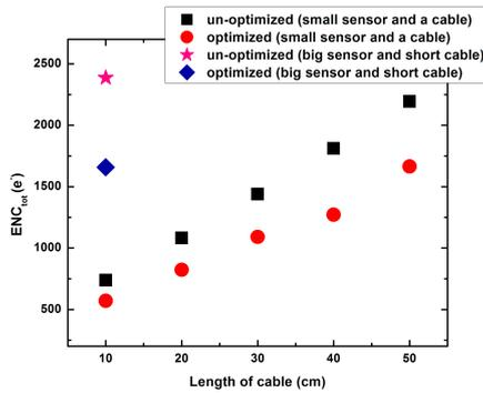
FIG. 1: Comparison of noise for the present prototype module and the optimized modules with new sensor (or detector) design and readout cables.
