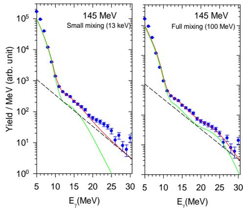
Fig.1. The experimentally measured  $\gamma$ -ray spectrum (filled circles) from  $^{32}\text{S}$  at  $E_{\text{lab}} = 145$  MeV. The CASCADE predictions using different mixing and GDR strength function is also shown along with the bremsstrahlung component (dashed lines).
