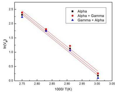
**Fig.1:** Variation of bulk etch rate ( µm\h) with temperature for alpha, alpha+gamma, and gamma+alpha irradiated CR-39 detectors.
