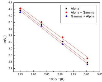
**Fig.2:** Variation of track etch rate ( µm\h) with temperature for alpha, alpha+gamma, and gamma+alpha irradiated CR-39 detectors.
