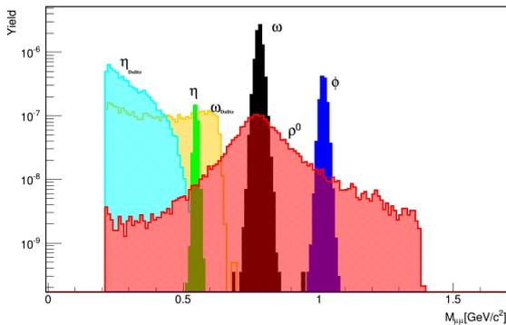
Figure 4: Invariant mass distributions of reconstructed muon pairs from decaying sources of cocktail for central Au+Au collisions at 25 A GeV
