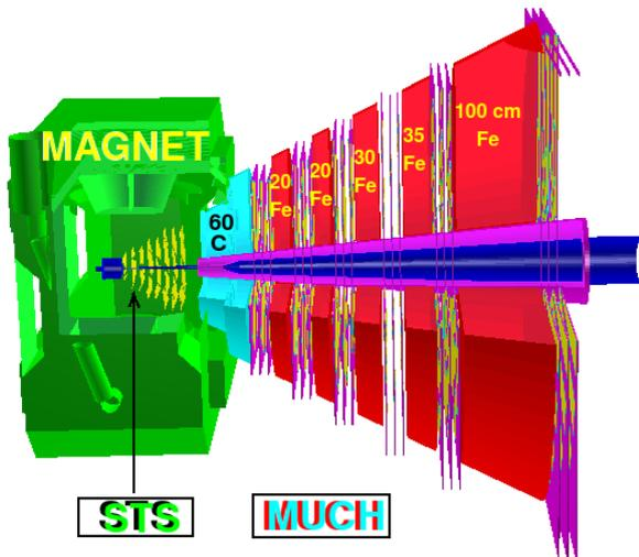
Figure 1: Muon Chamber set-up in CBM experiment for 25 AGeV collision energy
