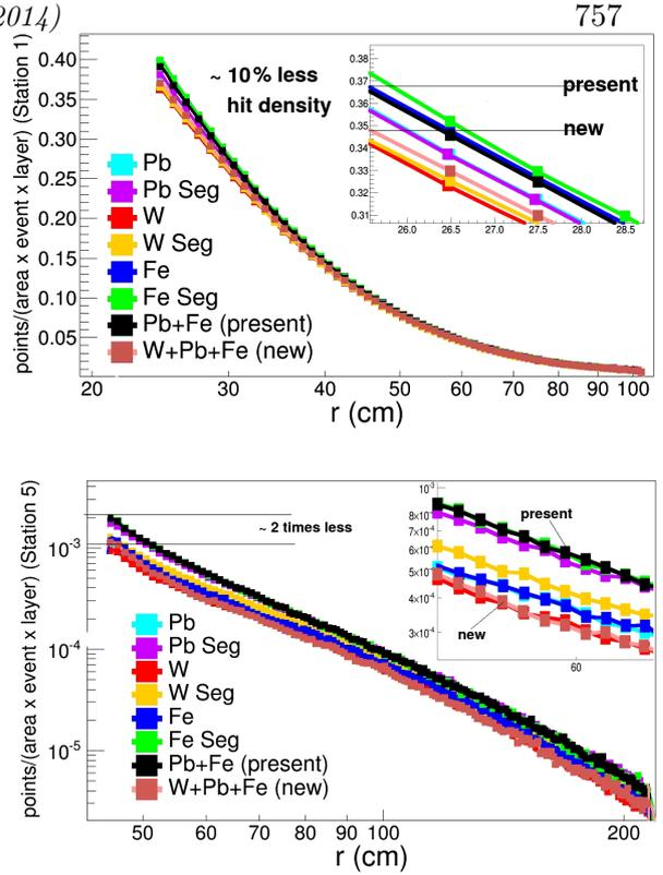
Figure 3: Point/Hit density at: Detector Station first (upper panel) and Detector Station fifth (lower panel) of MUCH for different beam-pipe shielding materials at 25A GeV central Au+Au collisions
