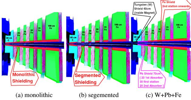
Figure 2: Muon Chamber with (a) Monolithic, (b) Segmented, and (c) New Optimised Combination [W(40cm) + Pb(70cm) + Fe(335cm)] beam-pipe shielding set-up for 25A GeV central Au+Au collisions
