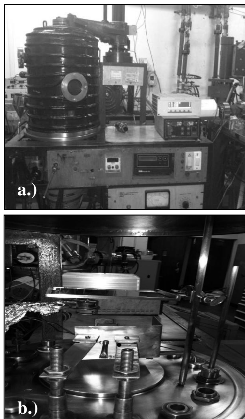
Fig. 1 High Vacuum Evaporator: a.) Outer view, b.) View inside the chamber.
