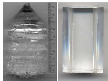
Fig. 1 As-grown single crystal and hexagonal shaped scintillator cut from the ingot.
