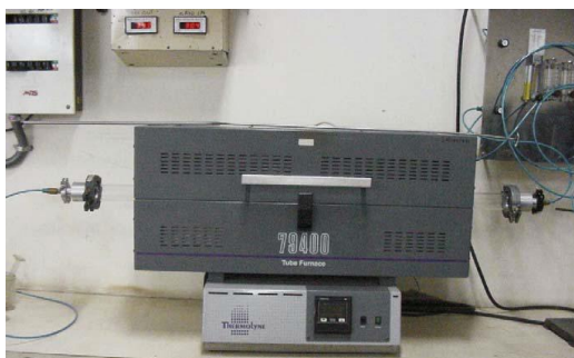
Fig. 2 Front view of the tube furnace used for annealing of carbon glass slides.
