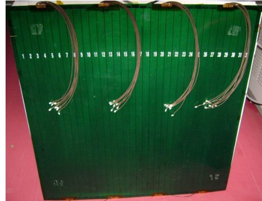
Figure 1: 1 m x 1m G-10-Readout with 32 read out strips (strip dimensions: 3 cm x 100 cm)
