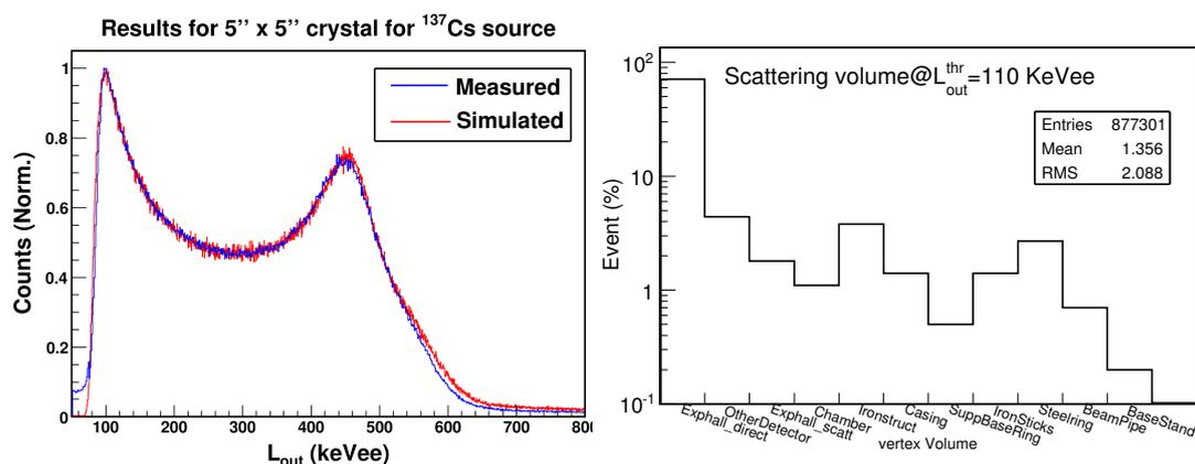
FIG. 1: Comparison between simulated and experimental light output (left), scattering volume distribution of the full array events at 110 keV light threshold for <sup>252</sup>Cf source.
