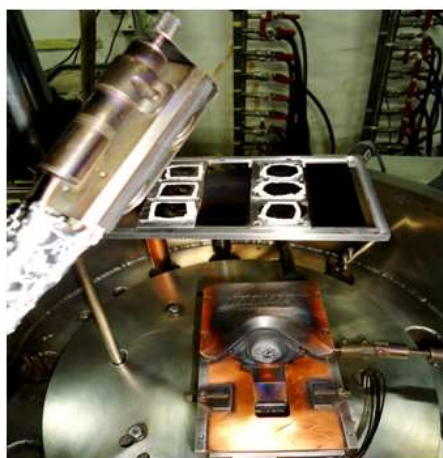
FIG. 2: Set-up for Ta deposition.
