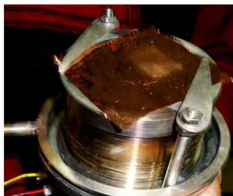
FIG. 1: Rolled copper foil fixed on the substrate heater.
