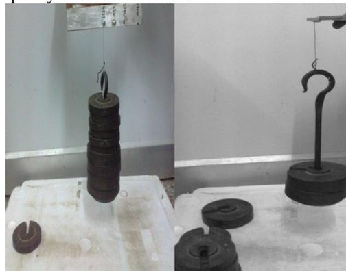
**Fig. 1** Pulling in horizontal direction and vertical direction of soldered wire (from left to right)
