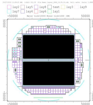
**Fig. 1:** Layer-wise mask image for detector development in kLayout software
