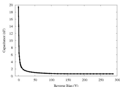
**Fig. 3:** CV measurement of one of the fabricated detectors.
