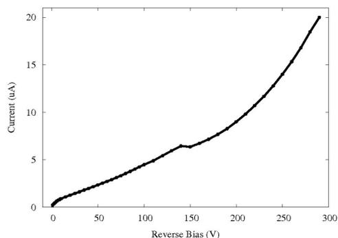
**Fig. 2:** IV measurement of one of the fabricated detectors.
