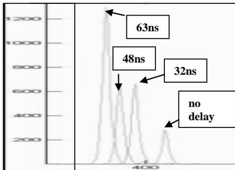
**Fig. 2** Shift in peak positions with varying delay
