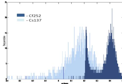
**Fig. 3** Overlapping PSD histograms generated with events from <sup>137</sup>Cs and <sup>252</sup>Cf source
