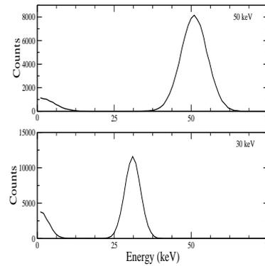
FIG. 2: The GEANT4 simulated spectra for 50 (top) and 30 keV (bottom) gamma-rays.
