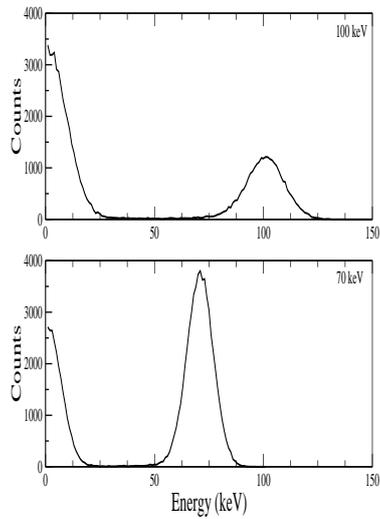
FIG. 1: The GEANT4 simulated spectra for 100 (top) and 70 keV (bottom) gamma-rays.
