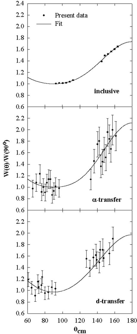
FIG. 1: Fission fragment angular distributions for reaction  ${}^6\text{Li} + {}^{238}\text{U}$  at energy  $E_{beam} = 36$  MeV for (a) inclusive (total-fusion fission) (b)  $\alpha$ -transfer and (c) d-transfer. Solid lines correspond to the fit to data to obtain FF angular anisotropy.
