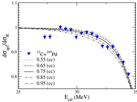
FIG. 1: Comparisons of the coupled-channel calculations for the quasi-elastic excitation function obtained with several values of the surface diffuseness parameter,  $a_0$ , in the nuclear potential for the  $^{12}\text{C} + ^{105}\text{Pd}$  system.
