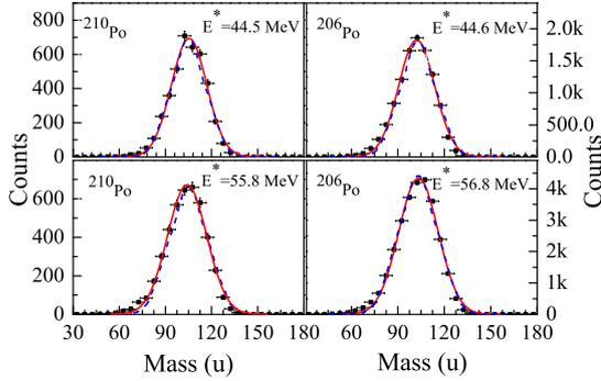
FIG. 1: Measured of fragment mass distributions at different excitation energies. Single Gaussian fits are shown by solid (red) lines. Theoretical fits are shown by the dashed (blue) lines.
