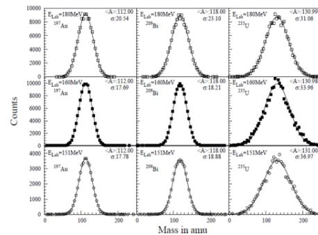
Fig.2. The mass distribution for various energies.
