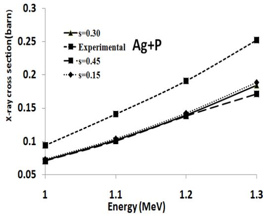
**Figure 2:** fig. shows K shell X-ray production cross section calculated for Ag target using low energy proton beam and compared with experimental data was taken from [1]
