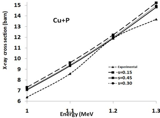
**Figure 1:** fig. shows K shell X-ray production cross section calculated for Cu target using low energy proton beam and compared with experimental data was taken from [1].
