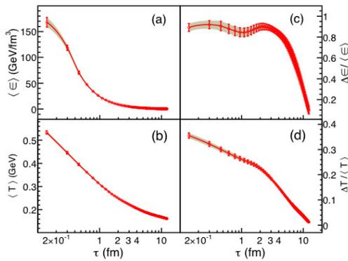
**Figure 2:** Temporal evolution of (a) average energy density, (b) average temperature, (c) fluctuations in energy density, and (d) fluctuations in temperature, for central Pb-Pb collisions at  $\sqrt{S_{NN}} = 2.76$  TeV, obtained from hydrodynamic calculations. The shaded region represents the extent of the event-by-event variations.
