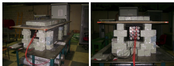
Fig. 1: Photographs of the prototype detector array for background studies with a matrix of 3 x 4 scintillators inside the lead shielding in the Dhruva reactor hall
