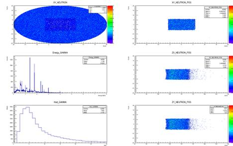
Fig2: Reconstructed image without any gamma energy or multiplicity selection.
