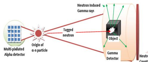
Fig. 1: Schematics of Simulated geometry for SNM detection
