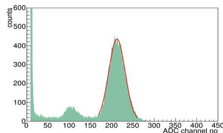
Fig.-1. The energy spectrum of Fe<sup>55</sup> X-ray source.
