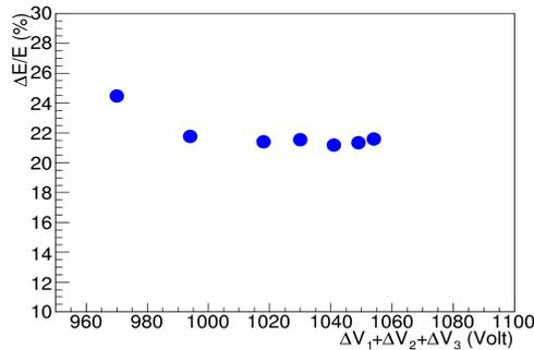
Fig.-3. Energy resolution as a function of global GEM voltage.
