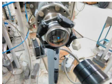
Fig. 3. Alignment testing by using the p beam of 3 MeV. From the figure we can see that the p beam having well focused (1mm) diameter has been achieved and very well focused by the quadrupole. The transmission of the beam from the switching magnet to the last FC was more than 95%.
