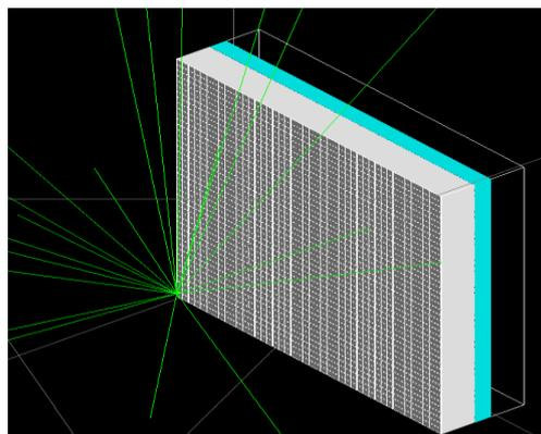
**Fig. 1:** Visualisation of the simulated gammas from a Co-57 source, interacting a collimator-detector geometry.
