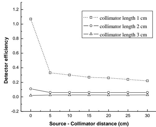
**Fig. 4:** Detector efficiency Vs. Collimator-source distance for different collimator length.
