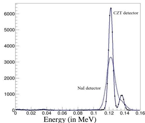
**Fig. 2:** GATE simulation of a Co-57  $\gamma$ -spectrum taken using a CZT and a NaI detector.
