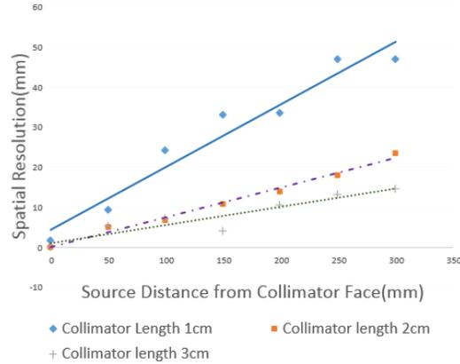
**Fig. 3:** Comparison of Spatial Resolution for different collimator lengths and different Source-Collimator distances.
