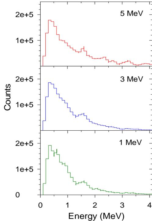
Fig. 3. Background-corrected pulse height spectra measured with the BaF<sub>2</sub> detector for three neutron energy bins for in beam experiment. The energy scale corresponds to electron-equivalent energy.
