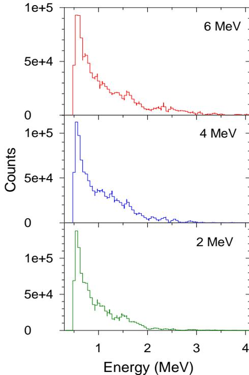
Fig.2. Background-corrected pulse height spectra measured with the BaF<sub>2</sub> detector for three neutron energy bins for <sup>252</sup>Cf source. The energy scale corresponds to electron-equivalent energy.
