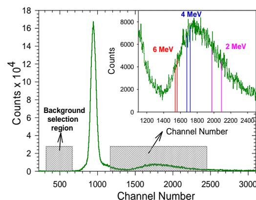
Fig. 1. The time of flight spectrum as obtained in one of the BaF<sub>2</sub> detectors using the <sup>252</sup>Cf source. The selection of the different energy regions in the TOF spectrum for generating the pulse height of particular energy is also indicated along with the area for background subtraction.
