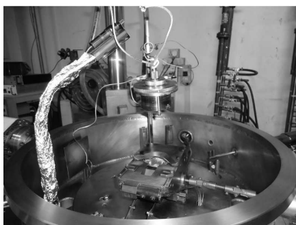
FIG. 2: Coating unit in an open position with a substrate heater above the crucible.
