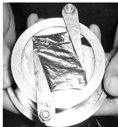
FIG. 3: Fabricated target placed on a substrate heater.
