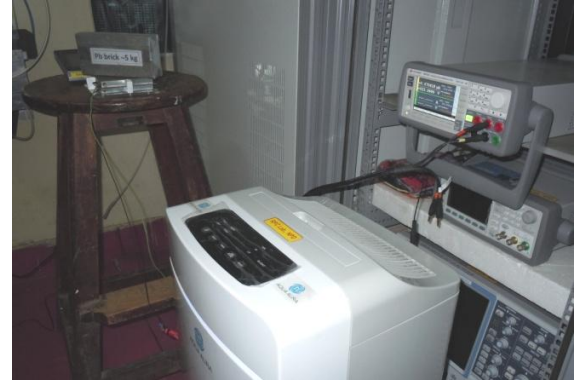
Fig. 2: The resistivity set up in RPC lab. (NPD)
