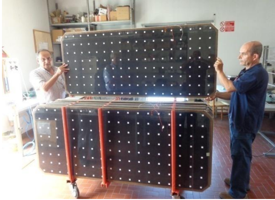
Fig. 1: Bakelite gas-gaps (1m x 2m) procured from GT, Italy
