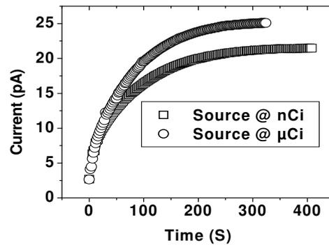
**Fig.3.** Same BOPET sample was exposed to 5 MeV  $\alpha$  from two different activity sources under vacuum and the device  $I-t$  curve was recorded.
