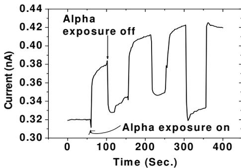
**Fig.1.** BOPET sample was periodically exposed to 5 MeV  $\alpha$  in air from a source of activity 0.5 mCi and the device  $I-t$  curve was recorded.
