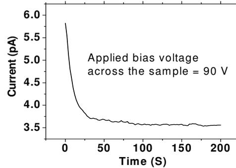
**Fig.2.**  $I-t$  characteristics of a BOPET sample in air prior to exposing it to an alpha source.
