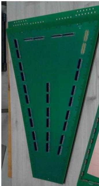
**Fig. 2** Bottom copper view of the readout PCB showing connectors for signal output from pads.
