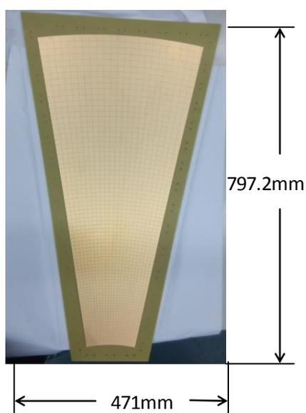
**Fig. 1** Top copper view of the readout PCB showing progressive geometry of the pads
