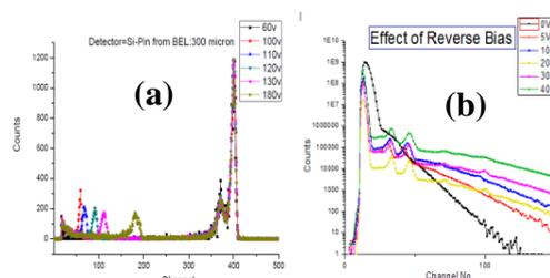
Fig. 2 The effects of increasing reverse bias on detection of (a) Electrons and alphas from <sup>241</sup>Am (b) X-ray and electrons from <sup>152</sup>Eu.
