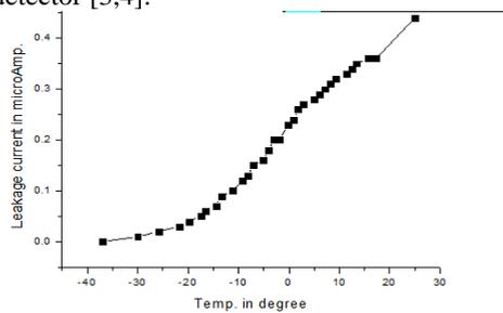
Fig 4 Variation of leakage current with temperature.
