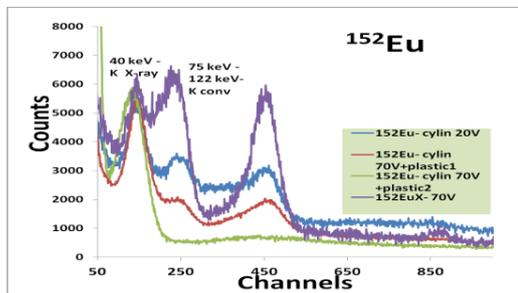
Fig. 3 The X-ray and conversion electron spectra
