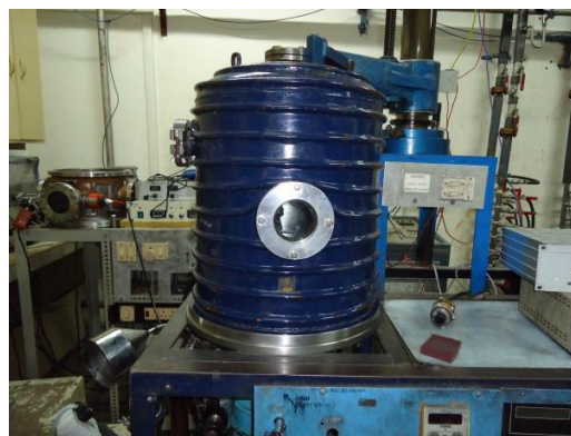
Fig.1. Outer view of High Vacuum Chamber at IUAC
